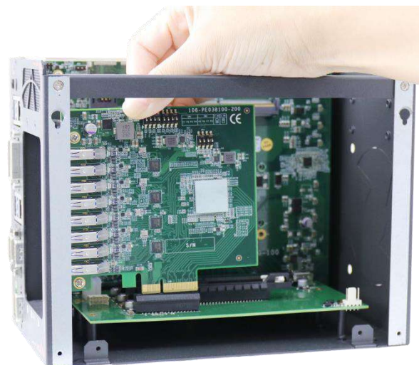
Insert gold finger into PCIe slot
