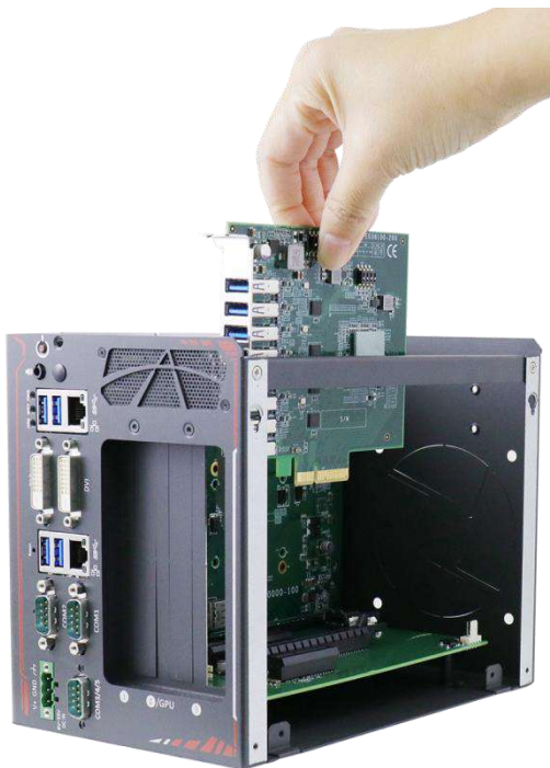
Lower PCIe-USB381F into the case
